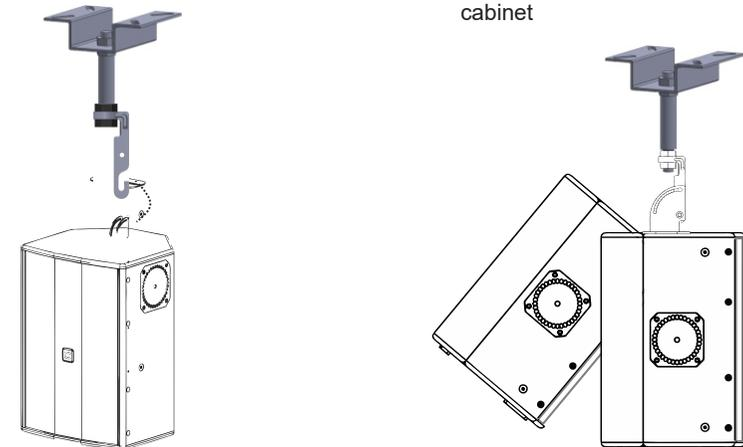
3. Install Speaker Bracket to the Screw Connector
