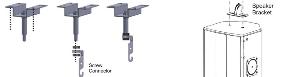
1. The Ceiling Bracket, attached to the Long Screw and then install bracket to the ceiling.
